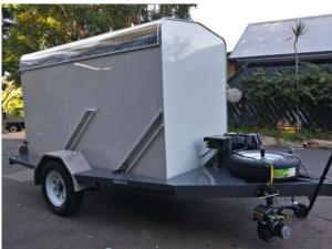
Using the remote control, you simply lower the trailer to the ground. Open the rear doors and wheel right on in. Tie down points are standard for securing your chair and load.
